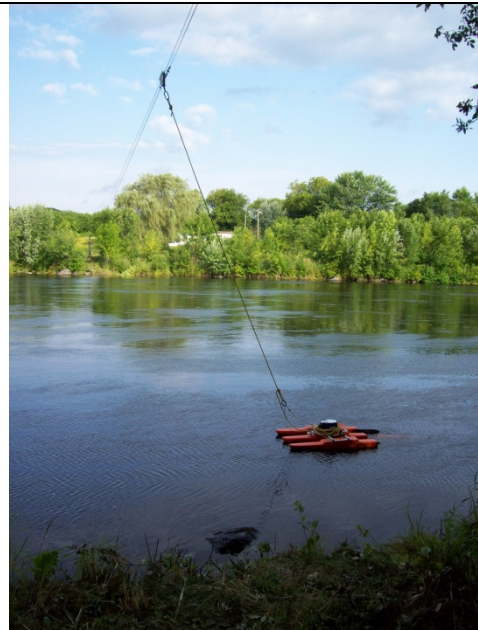
Acoustic Doppler Current Profile measurement using the bank operated cableway
