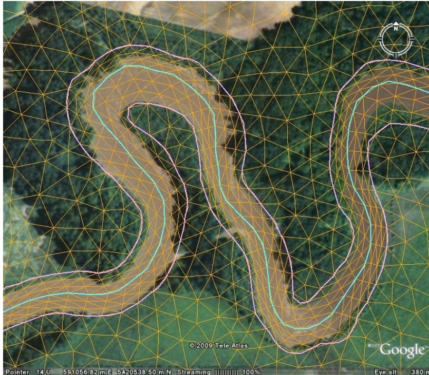
Figure 1 - Grid detail over a Google Earth aerial photo with top of bank lines and Thalweg
