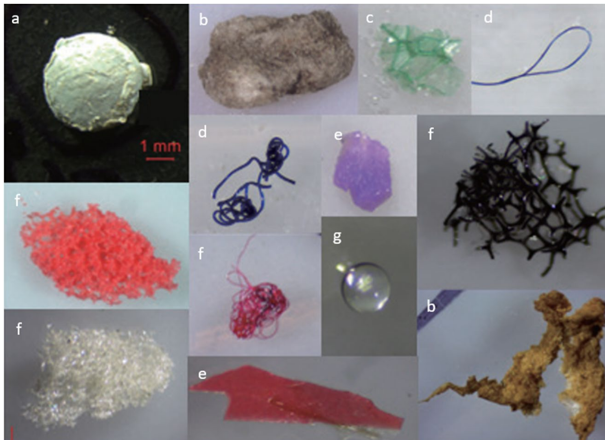
Figure 2-1: Microplastic Particle Morphologies Include (a) Pellets, (b) Foams, (c) Film, (d) Fibers, (e) Fragments, (f) Fiber bundles, and (g) Spheres. (Courtesy Martindale et al., 2020.)
