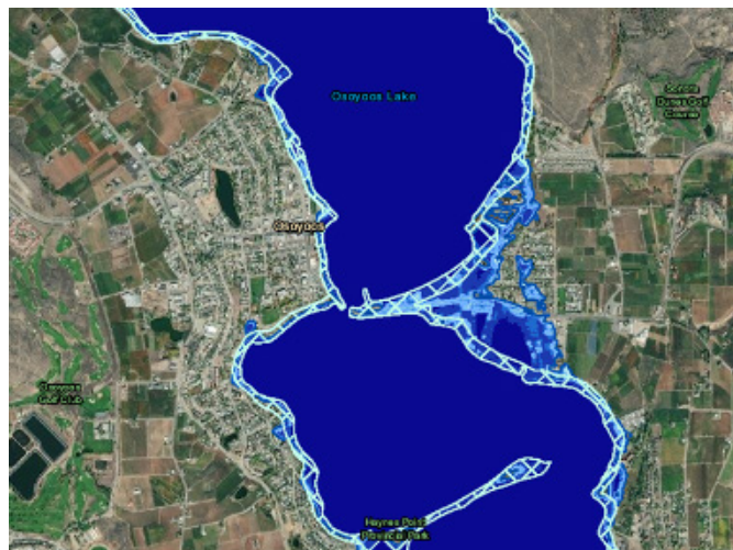
Figure 6. Osoyoos Lake Flood Construction Level (FCL) Zone (Inundation Extent). Example of 200-year design flood, gates open + mid-century climate change and freeboard. Source: Okanagan Flood Study. Northwest Hydraulic Consultants. 2022.
