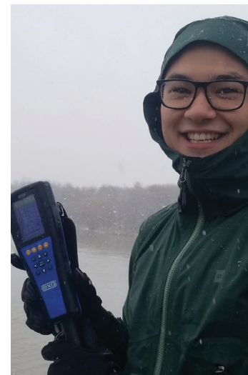
Staff using a water quality sonde to take a spot measurement.
