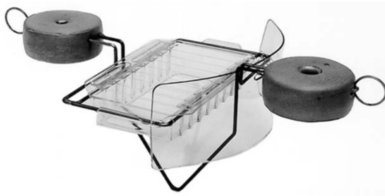
Figure 6-1. Floating Periphytometer Used at 30 Stations Within the Red River of the North During the Summer of 2015.
