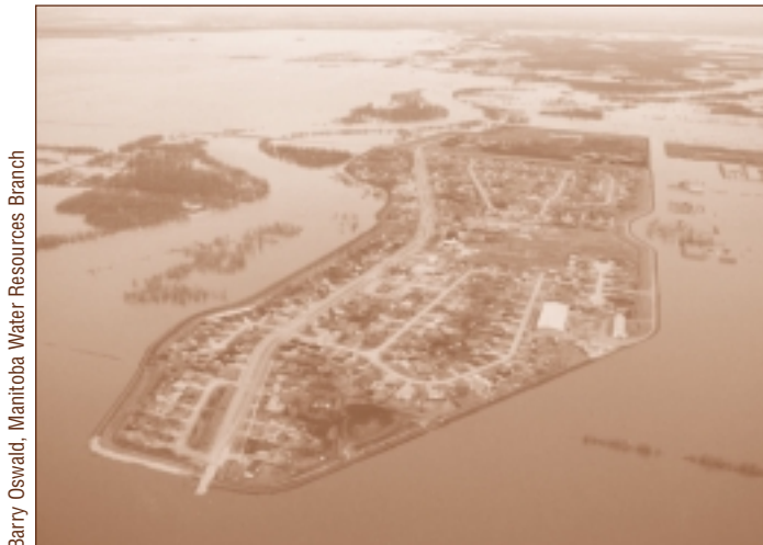
The ring dike surrounding St. Adolphe, Manitoba, holds back floodwaters, April 30, 1997.
