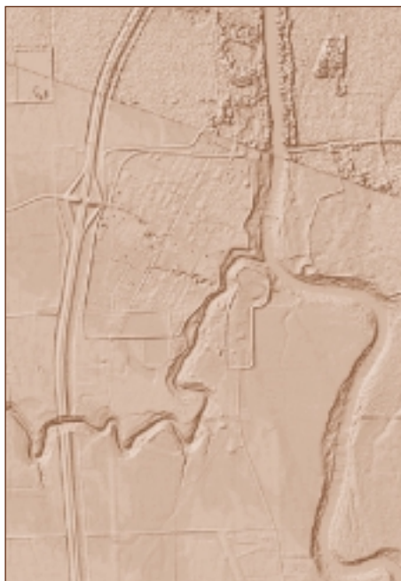
Fused imagery, Interferometric Synthetic Aperture Radar (IFSAR) with Light Detection and Ranging (LIDAR), shows topographic relief in the Pembina, North Dakota, area.
