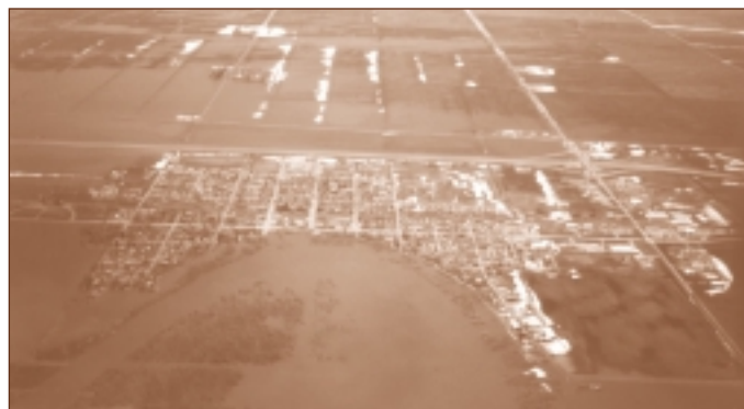
Raised roads near Drayton, North Dakota, capture floodwaters in a "waffle" pattern.
