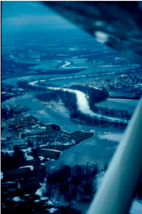
Figure 4. Red River breakup, April 13, 1989. Looking north toward Grand Forks, ND; flow is from bottom to top. The ice cover, comprising fractured sheet ice and occasional rubble, is contained in the channel by trees while the water is contained within the levees. Photo taken by Kathleen White, CRREL.
